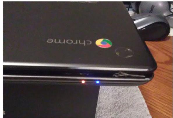
2. If there is a light but still no display, try pressing and holding the **Refresh** and **Power** keys shown below for 7 seconds. Then press the power button again. If there is still no display, this could be indicative of a possible hardware problem with the Chromebook.
